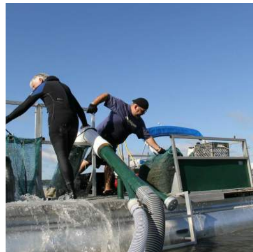
Diver Assisted Suction Harvesting (DASH).
